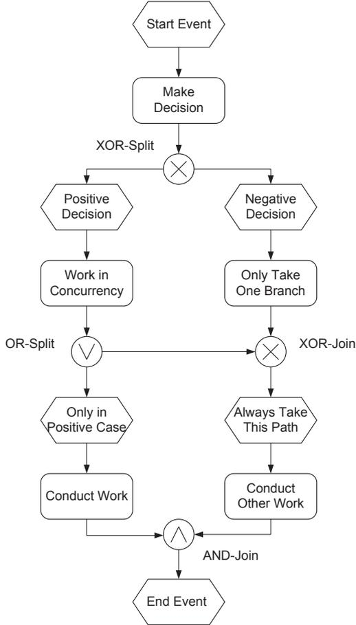
Figure 1: Example of an EPC process model
