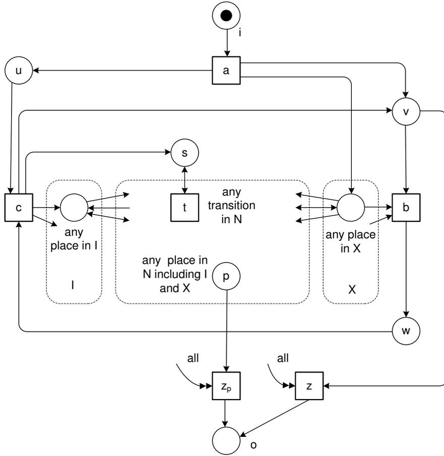
**Fig. 6.** Construction showing that soundness is undecidable for WF-nets with reset arcs. The original net comprises the three dashed areas:  $I$  is the set of places of  $N$  initially marked,  $X$  is the set of places that are marked in  $M_X$ , and all other nodes of  $N$  are shown in the dashed area in the middle. Note that  $I$  and  $X$  may overlap.
