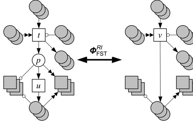
**Fig. 2.** Fusion of series transitions
