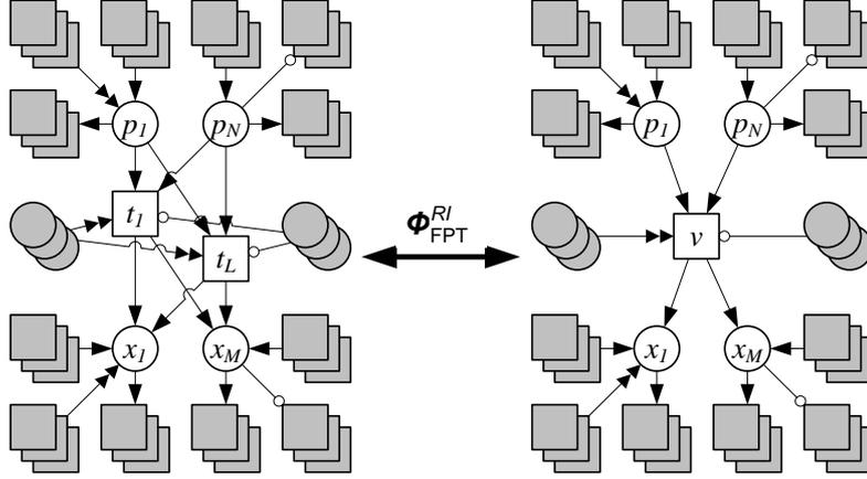
**Fig. 4.** Fusion of parallel transitions
