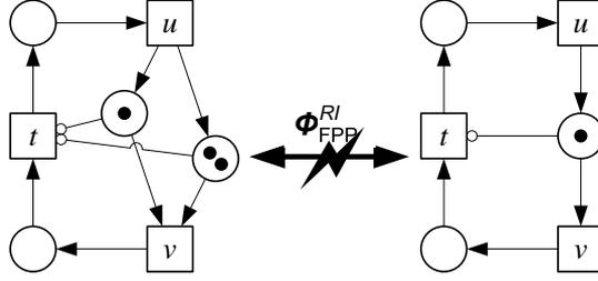
**Fig. 6.** Fusion of parallel places: Inhibitors explained
